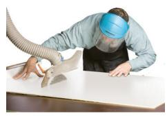
1. Using a suitable panel saw, cut StyleLite®, substrate and backing panel slightly oversize.
