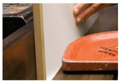
5. Trim laminated panels to final size using a plane or router.
