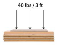
4. Laminate the 3 materials and press for a minimum of 4 hours with a moderate weight spread evenly across the panels. Overnight pressing is ideal.
